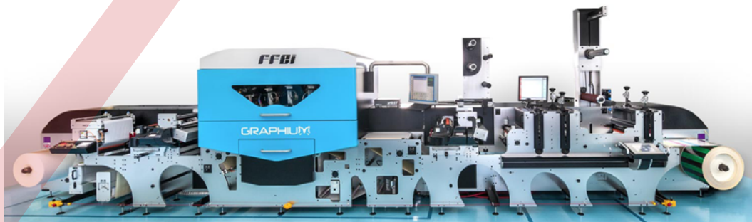
A Graphium UV press, combining flexo and digital inkjet. (Image courtesy of Fujifilm.)
