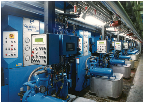
A TR 10B gravure press. (Courtesy Koenig & Bauer AG)
