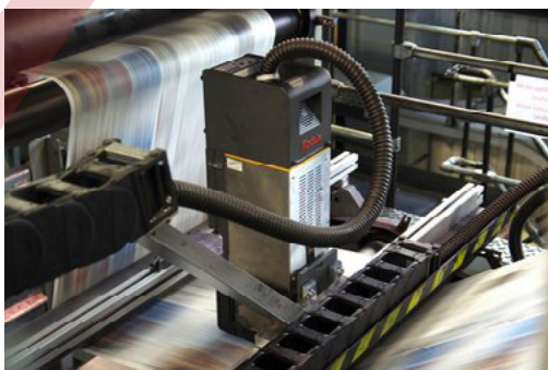
A Kodak Prosper inkjet head, combined with high-speed web offset to imprint each page with personalized information. (Image courtesy of Eastman Kodak.)
