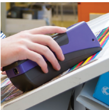
A densitometer measures the degree of darkness or light absorbance of a material—in this case a layer of ink or toner covering a substrate.
